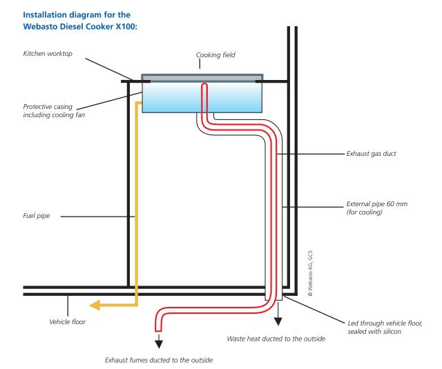
The cooker can be installed without difficulty in virtually all vehicles. The cooker is mounted from above into the recess in the kitchen worktop. A protective casing is fitted from below, and has an integrated cooling fan which ensures that the waste heat is ducted from the underside of the cooker to the outside via a flexible coaxial pipe.
